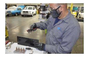
Mark the location of the rivets and types as per the OEM repair procedures.
