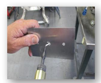
Remove E-coat from matting surfaces with scotch-brite disc or DA sander (low speed) with 80 grit or finer. Follow OE recommendations for this process.
