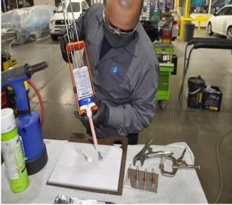
Apply adhesive to both mating surfaces, spread, cover all bare metal and apply another bead for a proper bond line thickness.
