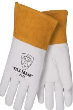
TIG welding gloves need more dexterity and finger sensitivity that MIG and Stick gloves because TIG is an intricate process. You'll ideally want gloves that are maneuverable but still provide adequate heat protection. It can be hard to hold a small welding rod with thick gloves, so TIG gloves usually use thinner materials such as goatskin, pigskin or deerskin. Having a thin lining or no lining will also help with dexterity. These gloves won't be suitable for Stick welding or MIG.
