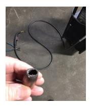
Check the nozzle on the gun for wear and if bad replace
