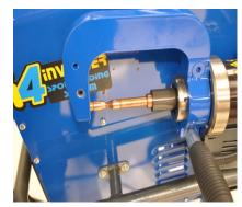
Align the tips using 3 set screws on the gun and recheck.
