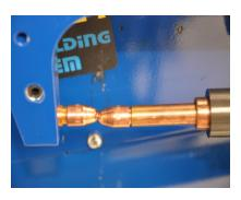
Check alignment on the tips. Note the tips in this scenario are not in alignment.
