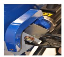
Use a shunt pliers for the first weld when weld bonding or leaving the E-coat intact between the mating surfaces.
