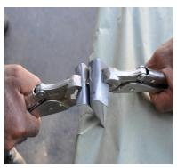
Perform a destructive weld test using same metal from the vehicle (See Best Practice for Testing Spot welds for procedures).
