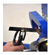
• Perform the weld. Remember to do the following: Place insulated clamps near the area that is being welded. Do not use the pressure from the gun to draw the flanges together. Finally, pull the gun so that the stationary electrode is making contact with the flange and the moveable electrode is driven into the flange.
