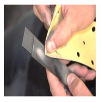
Clean the both outer flanges at weld site where the electrodes will make contact.
