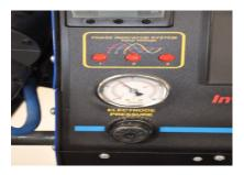
Set Air pressure for 90psi for standard gun (blue cover) and 50psi for high pressure gun (black cover).
